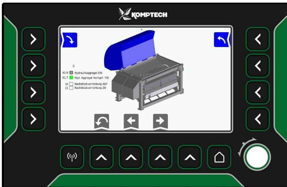
Fig. 30: Regim manual unitate de compactare
